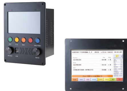
CCP (Communication Control Panel)
